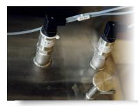
Indication of full or empty status with high/low fail safe limit switches can be done with NIVOSWITCH RCM-401-3 or NIVOSWITCH RFM-401-0 type vibrating fork level switches. Recommended multipoint temperature transmitter is THERMOPOINT TMM-5□□-5Ex type with HART® output. The measured values and alarms can be displayed on a MultiCONT PRW multichannel controller or on PC through UNICOMM SAK-305 HART®-USB/RS485 modem.
