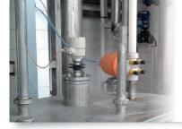
Continuous level measurement of the mixing tanks can be done with MicroTREK HHQ-413-4 type guided microwave level transmitters. Types with different process connections and fully PFA coated probes are available to satisfy food industry's high hygienic requirements. After mixing the liquid is transferred to the dosing machine and then dosed into the cans.
