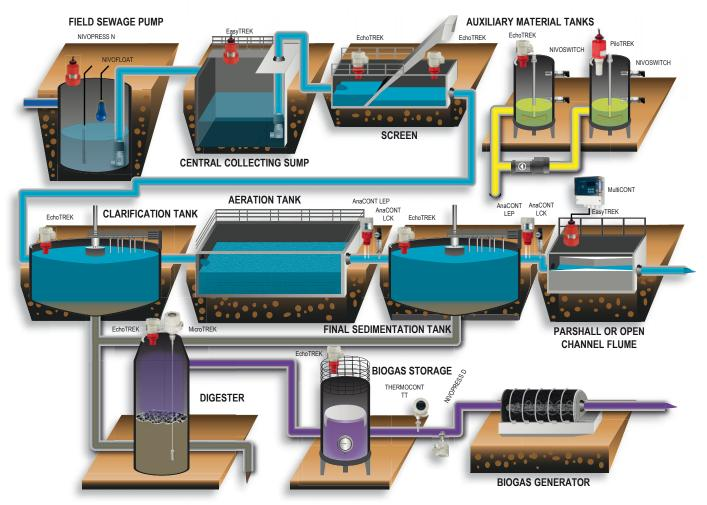
Sewage treatment can be divided into 2 major parts: field sewage collection and pumps, and the central sewage treatment facility. The sewage treatment process also has 2 separate sections: water treatment processes and slurry treatment processes.
